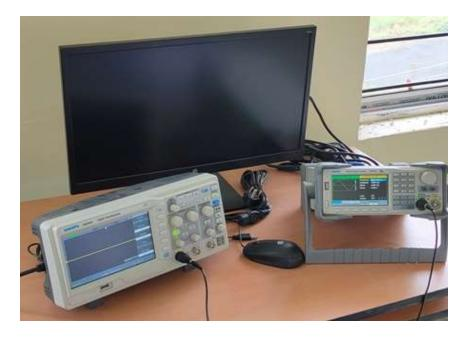
Laboratory experiments will be performed on oscilloscope, previously called an oscillograph, and informally known as a scope or o-scope, CRO (for cathode-ray oscilloscope), or DSO (for the more modern digital storage oscilloscope), is a **type of electronic test instrument that graphically displays varying signal voltages.**
